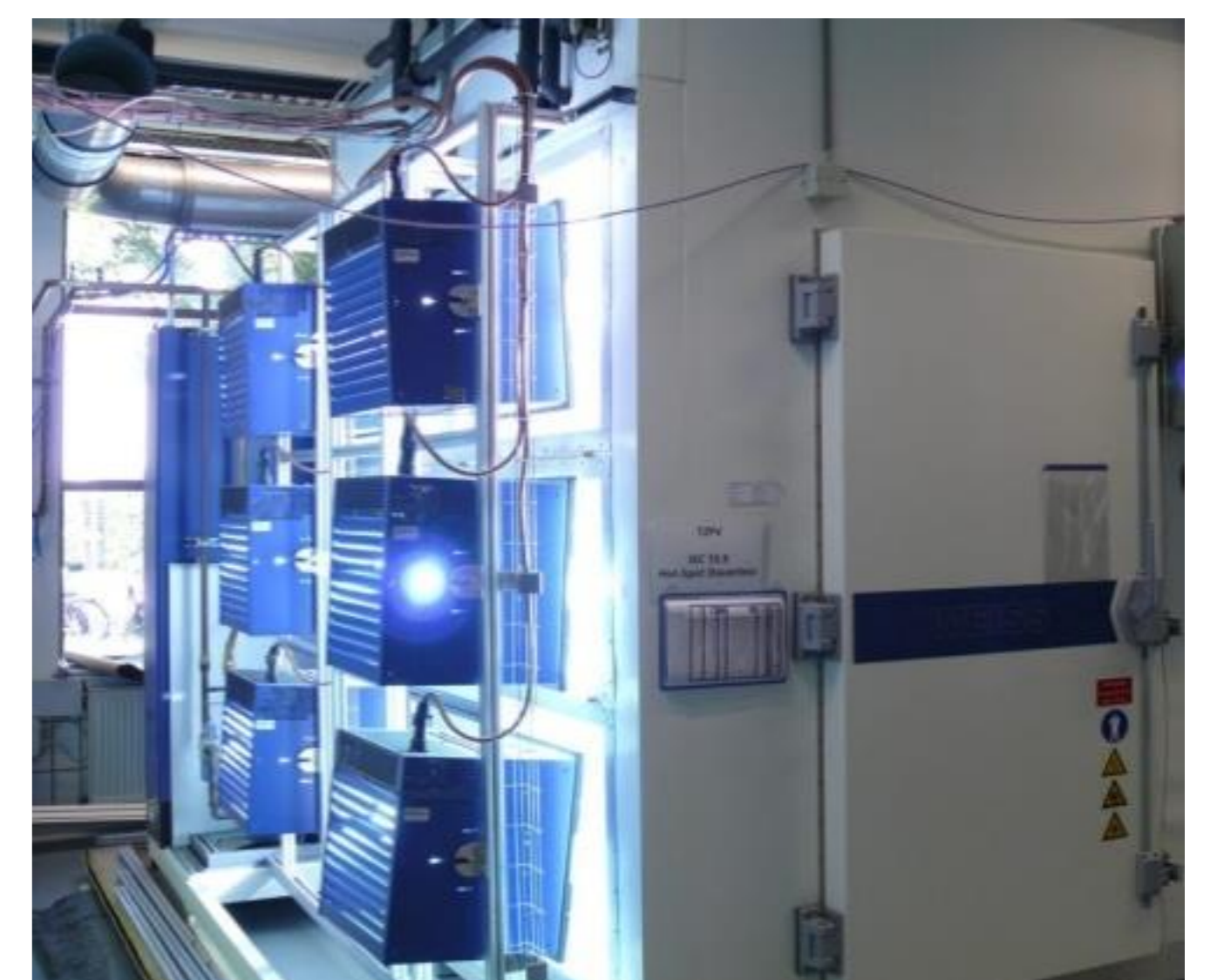
Climate chamber with combined light / temperature stress
