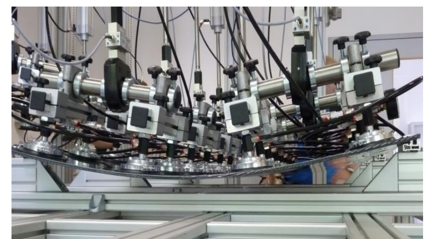
Mechanical load test of PV module
