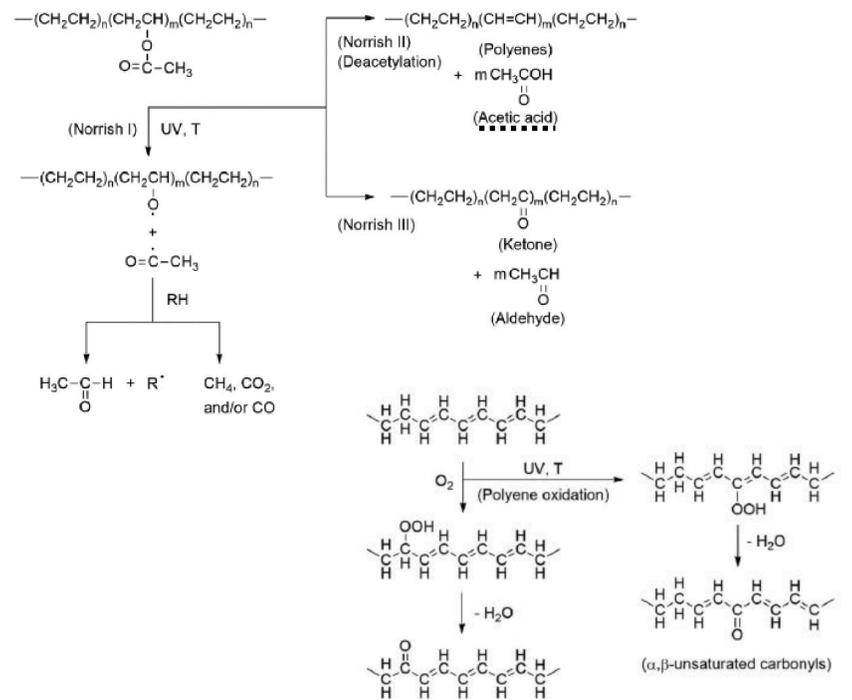
The degradation mechanism of EVA is characterized by the initial de-acetylation and the production of acetic acid and polyenes because of thermal energy and radiations, according to the Norrish II reaction.
