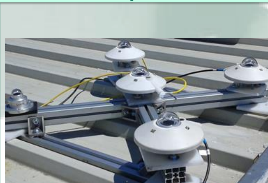
Outdoor calibration of pyranometers [image kindly provided by EURAC]
