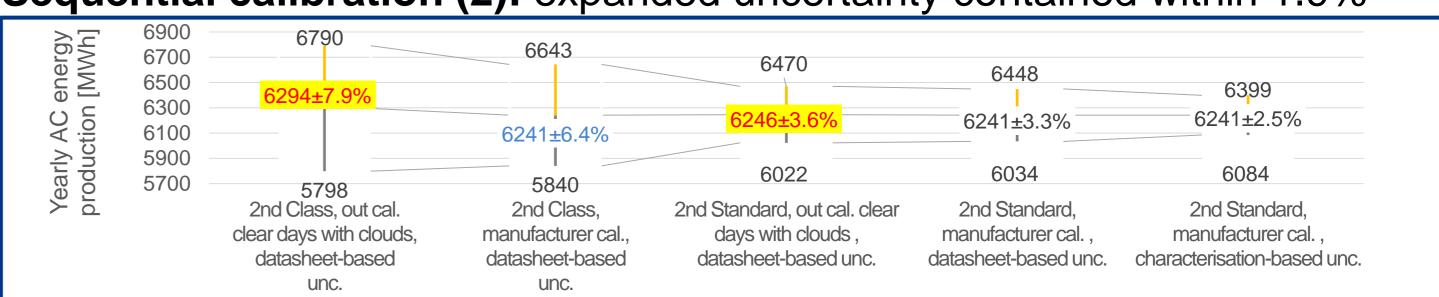
Scenarios evaluation (3): expanded uncertainty up to 7.9% (496 Mwh) and 3.6% (224 Mwh) for 2C and SS in annual yield of PV solar farm of 7.4 MWp
