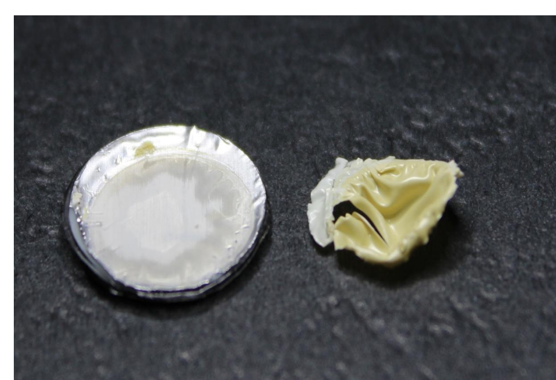
Delaminated and degraded PA-ALU backsheet.
