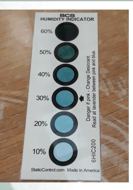
The humidity indicator cards include dots constructed from blotting paper impregnated with cobaltous chloride, which is sensitive to moisture. Each dot has a different concentration of cobaltous chloride and is designed to indicate a different level of humidity [1].
