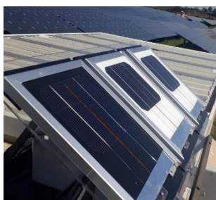
Outdoor monitoring setup of moisture ingress installed in Rome
