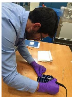
**Soldering of a solar cell metallization**
